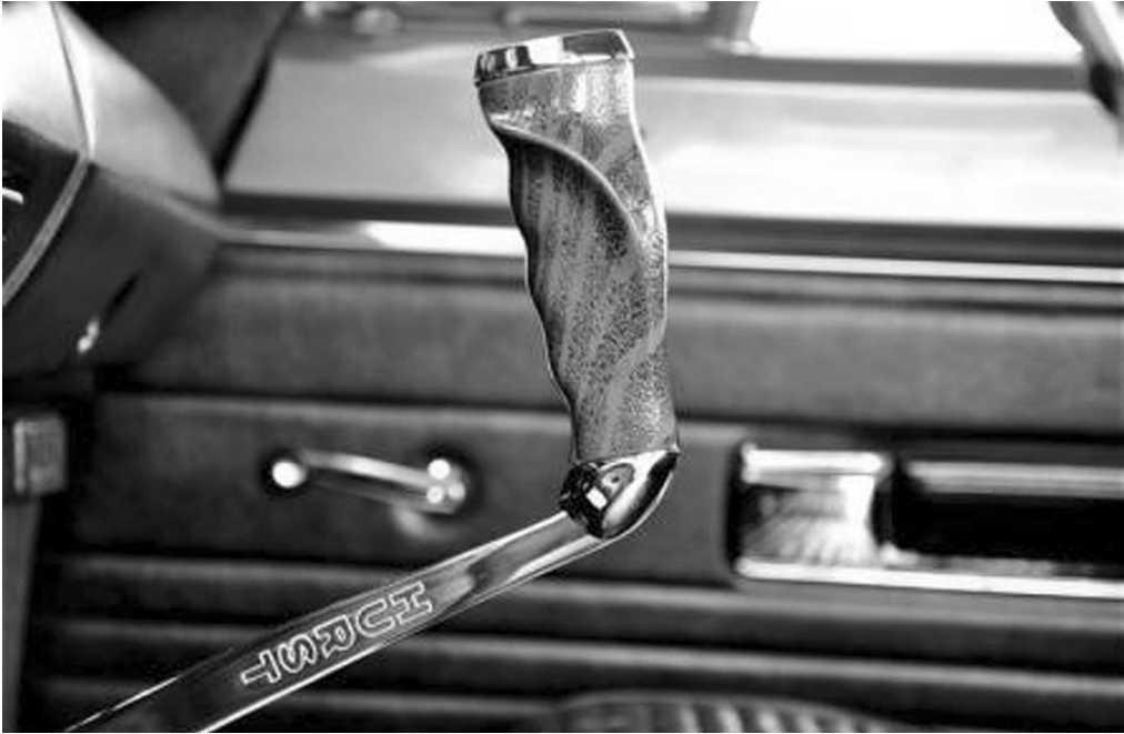
One of Chrysler's most memorable features of the muscle car era, the Hurst "Pistol-Grip" shifter (courtesy Steven Anastos, Red Hills Rods and Classics, St. George, UT).
